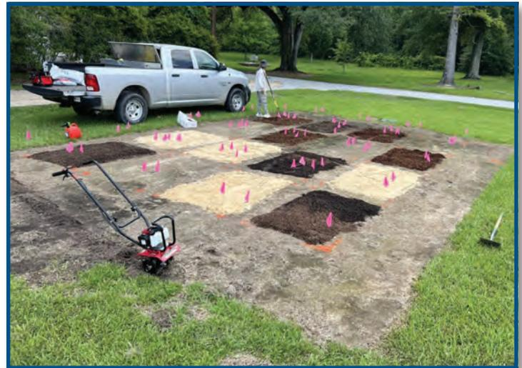
Photo 1. The purpose of this research was to determine the effect of soil amendments on root morphology, soil volumetric water content, and turf visual quality after establishment of centipedegrass sod. In this photo, soil amendments were applied across all plots.
